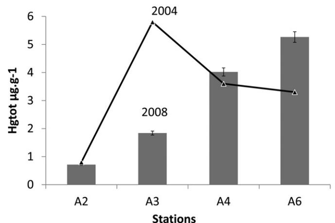
**Fig. 3.** Comparison of Hg-T in this study (gray histograms), sampling period 2008; bars indicate standard deviation of triplicate analyses. Hg-T determined in sediments of same stations in 2004 (continuous line), data from Covelli et al. (2009).
